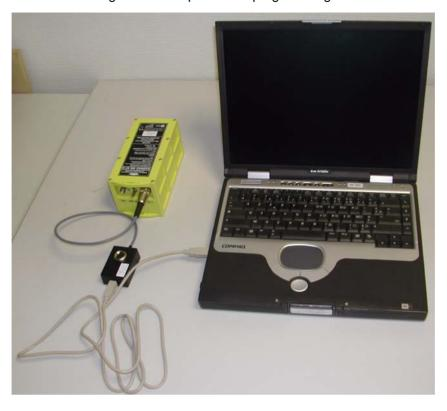
Figure 3: Example of ELT programming with PR600
